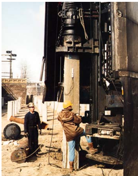
Fig 9. Dynamic load test on a precast pile
