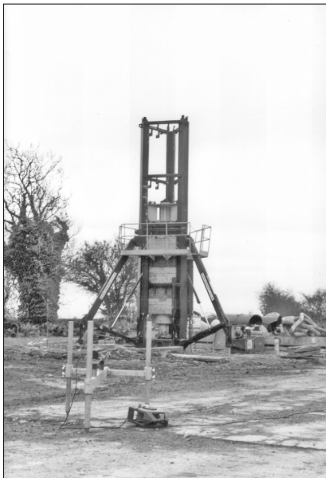
Fig. 1. 3 MN Statnamic device with hydraulic catch mechanism. The laser reference source can be seen in the foreground
