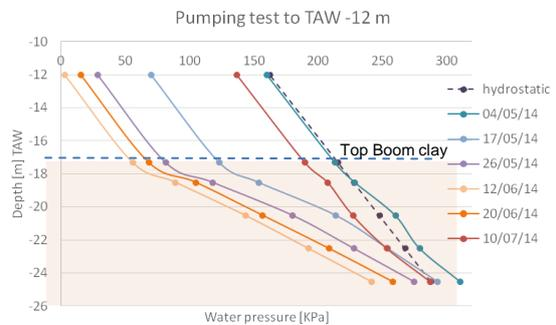
Figure 9. Pore pressures Boom clay during pumping test
