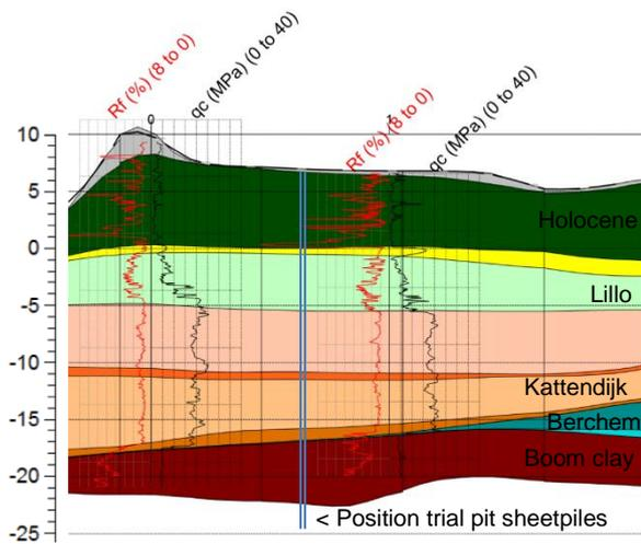
Figure 4. Soil strata at the trial pit location
