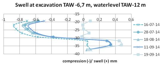
Figure 12. Vertical effect per module excavation -6.7 m
