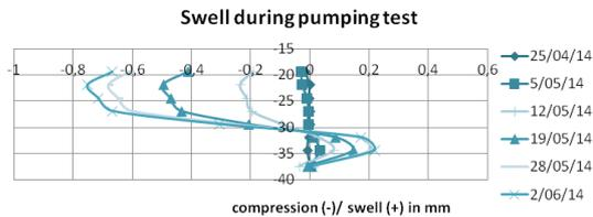
Figure 11. Vertical effect per module pumping test
