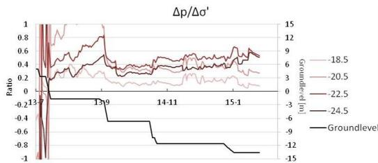
Figure 15. Transfer ratio pore pressure / effective stress
