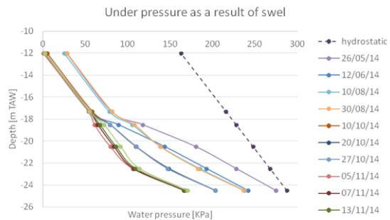
Figure 10. Pore pressures Boom clay during excavation
