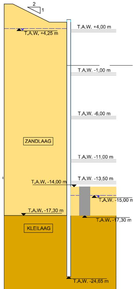
Figure 5. Cross-section trial pit at TAW -14 m excavation
