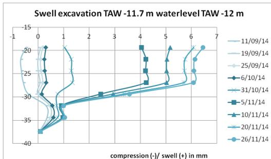
Figure 13. Vertical effect per module excavation -11.7 m
